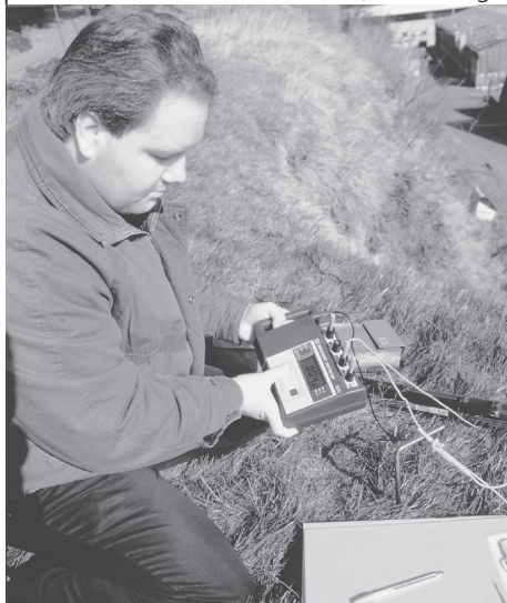
Typical use of a Megger digital ground resistance tester to perform fall-of-potential testing
